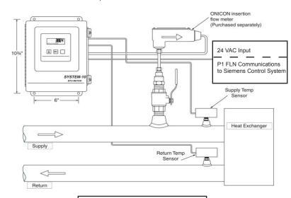
Insertion turbine flow meter shown. Any ONICON flow meter may be used with the System-10 BTU Meter. Consult with ONICON for additional flow meter types.
