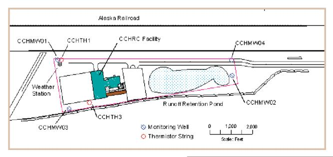
Figure 1. Site location map for CCHRC facility showing location of observation wells and thermistor borings. Locations of wells and thermistor strings are approximate.
