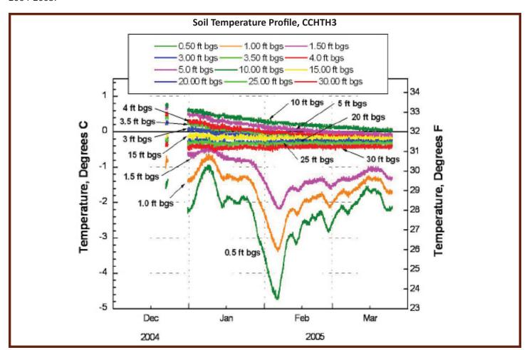
Figure 2. Site CCHTH3, located on the southwest side of the CCHRC property. All thermistor readings are shown with depth labels. Installation occurred on 12/9/04.
